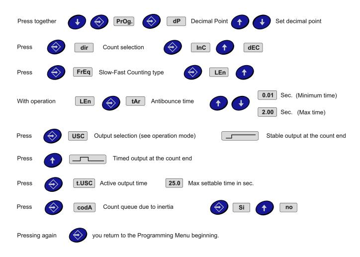
If after 5 seconds no operation is carried out, the instrument will automatically exit the Programming, storing all the set Parameters.
